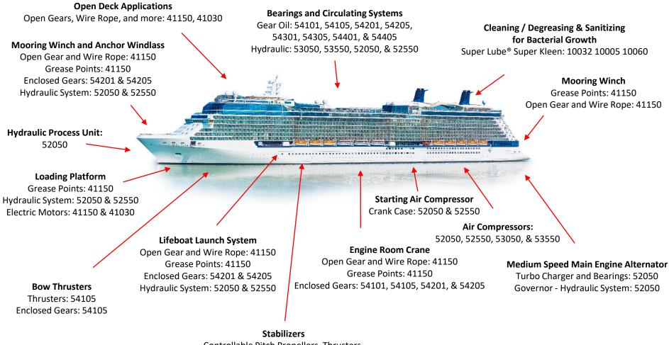
Controllable Pitch Propellers, Thrusters, Propulsion Drives, & Certain Tube Designs: 53050, 53550, 52050, & 52550
